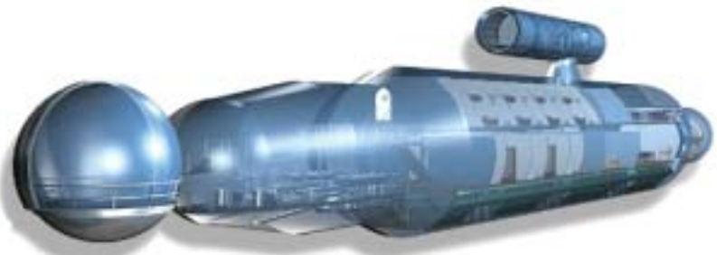
The pressure hull viewed from aft. The spherical diver lock-out chamber also has a dry transfer lock for entering the submarine at the top.
