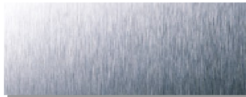
2K This smooth reflective surface makes it particularly suitable for most architectural applications, especially exteriors where atmospheric performance is critical. The finish is obtained by the use of finer grit belts or brushes which give a clean cut finish with a roughness of R_a = 0.5 microns maximum.
