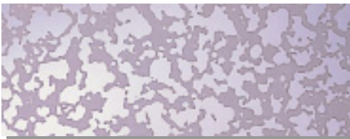
The depth of etching is controlled by the length of time that the stainless steel is exposed to the acid.
